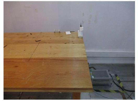
7.2 Radiated Disturbance(30MHz-1GHz) Test Setup
