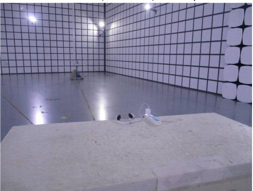
7.1 Radiated Disturbance(30MHz-1GHz) Test Setup
